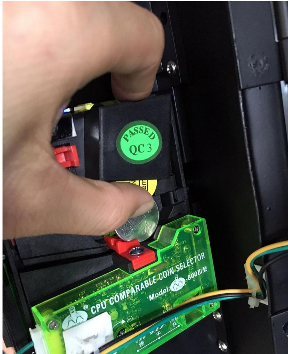
1) If put \$1 coin in this place, then the coin acceptor can accept \$1 coin.
